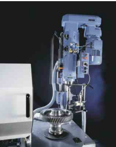
New, VM machine with drill correction
