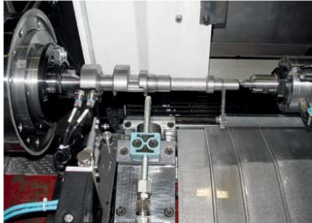
Peel grinding combines the durability and efficiency of CBN wheels, with the process advantages of high-speed grinding.
