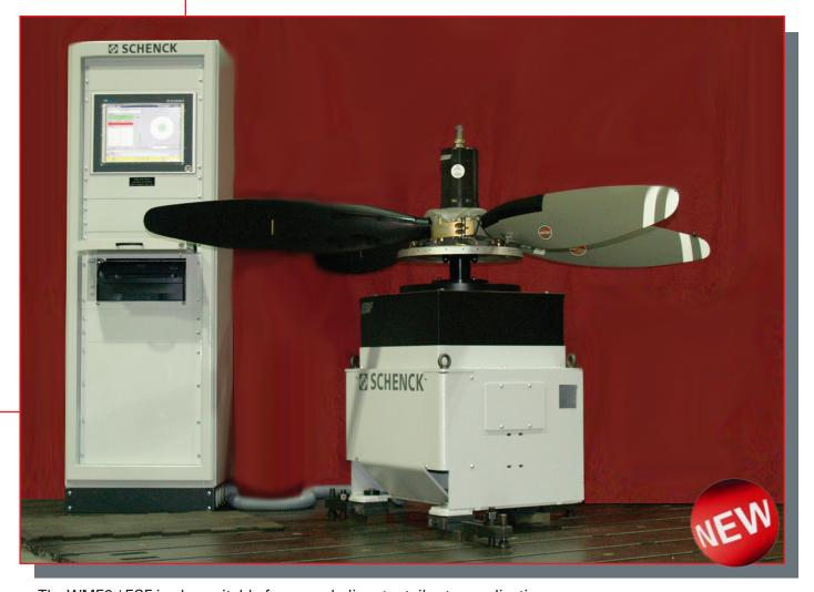
The WME3 / ESF is also suitable for many helicopter tail rotor applications. Contact Sales@Schenck-usa.com for more information.
