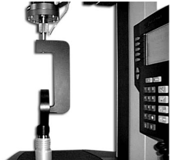
▲ Gooseneck extension for ease of internal testing.
