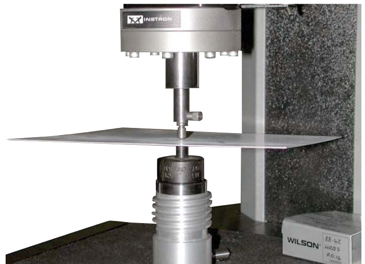
▲ Wilson® Rockwell®2000 series tester performing hardness test on sheet using diamond spot anvil.
