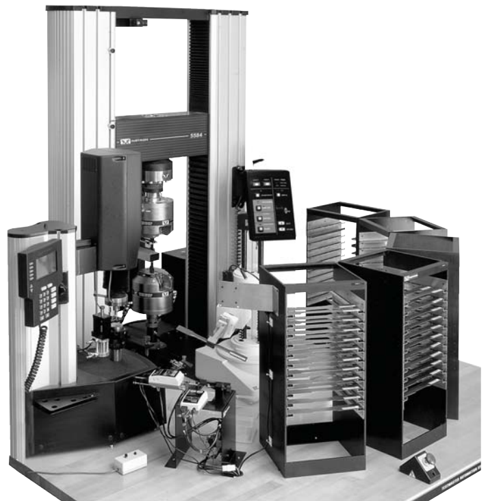
▲ Rockwell series 2000 tester integrated with Instron® universal test system designed for automatic loading and testing with a robot.
