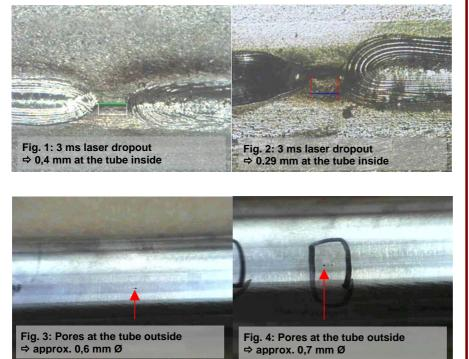
Laser welded stainless steel tubes
