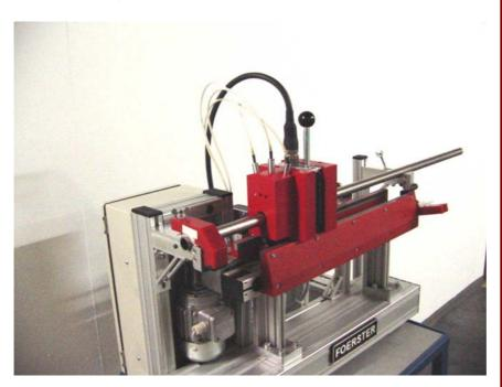
This is realised by setting up two test stations, one station equipped with a sensor array, the second station with an encircling coil. Each station works with separate signal recording up to the sorting and / or marking stage. The results of both stations are collated again for the report and for data saving.
